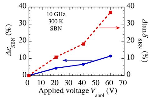
Evolution as a function of applied bias, of relative variations of the dielectric permittivity (blue) and of the loss tangent (red) for a 500 nm thick SBN film at 10 GHz and 300 K
