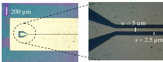
Photos with microscope of a Au/SBN/MgO transmission line of 5  $\mu\text{m}$  width.
