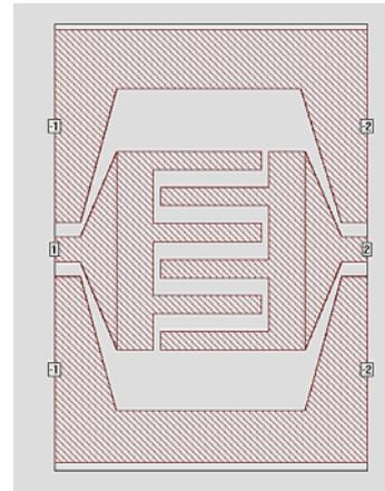
Schematics of an interdigital capacitor simulated by Sonnet®
