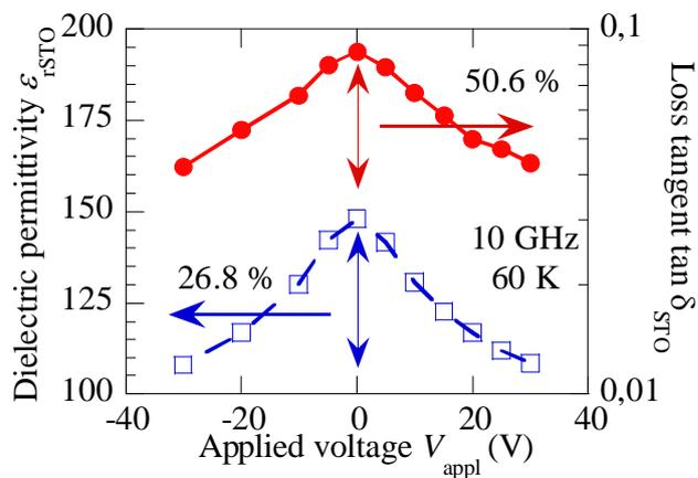
Evolution as a function of applied bias, of dielectric permittivity (blue) and of the loss tangent (red) for a 250 nm thick SrTiO<sub>3</sub> film at 10 GHz and 60 K. The relative variation is given in percent.
